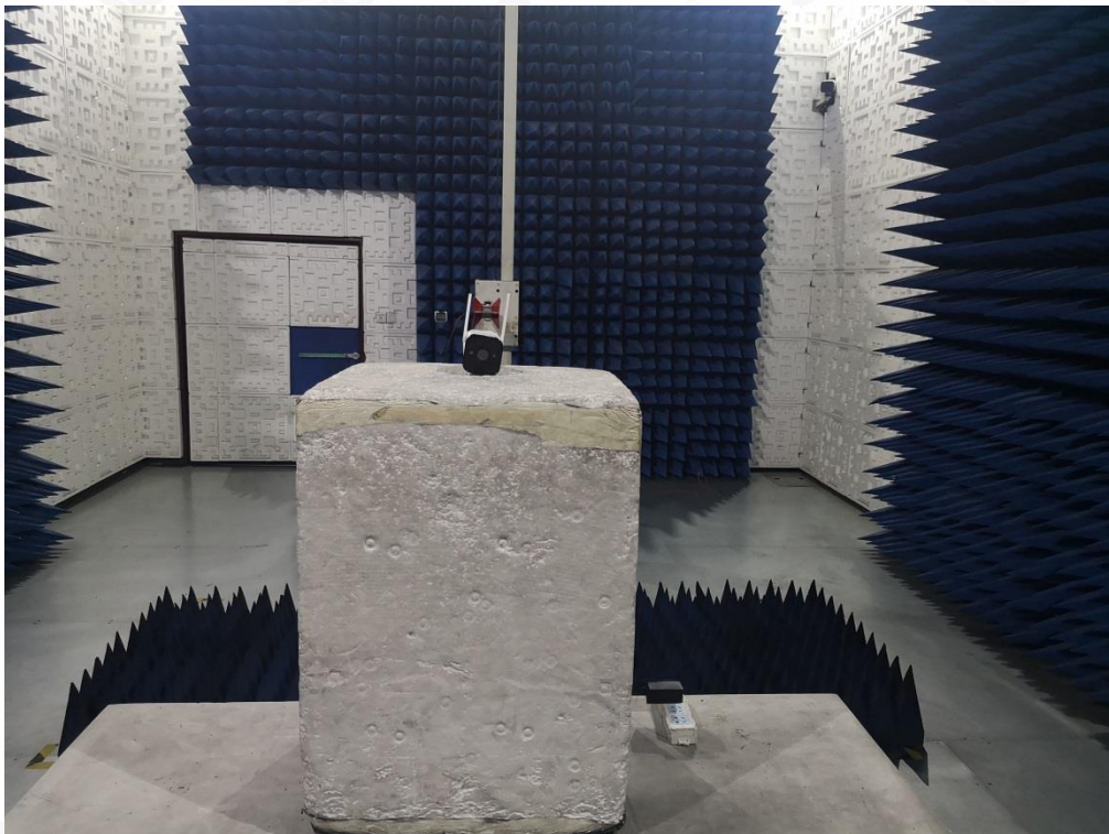
FCC RADIATED EMISSION TEST SETUP ABOVE 1GHZ
