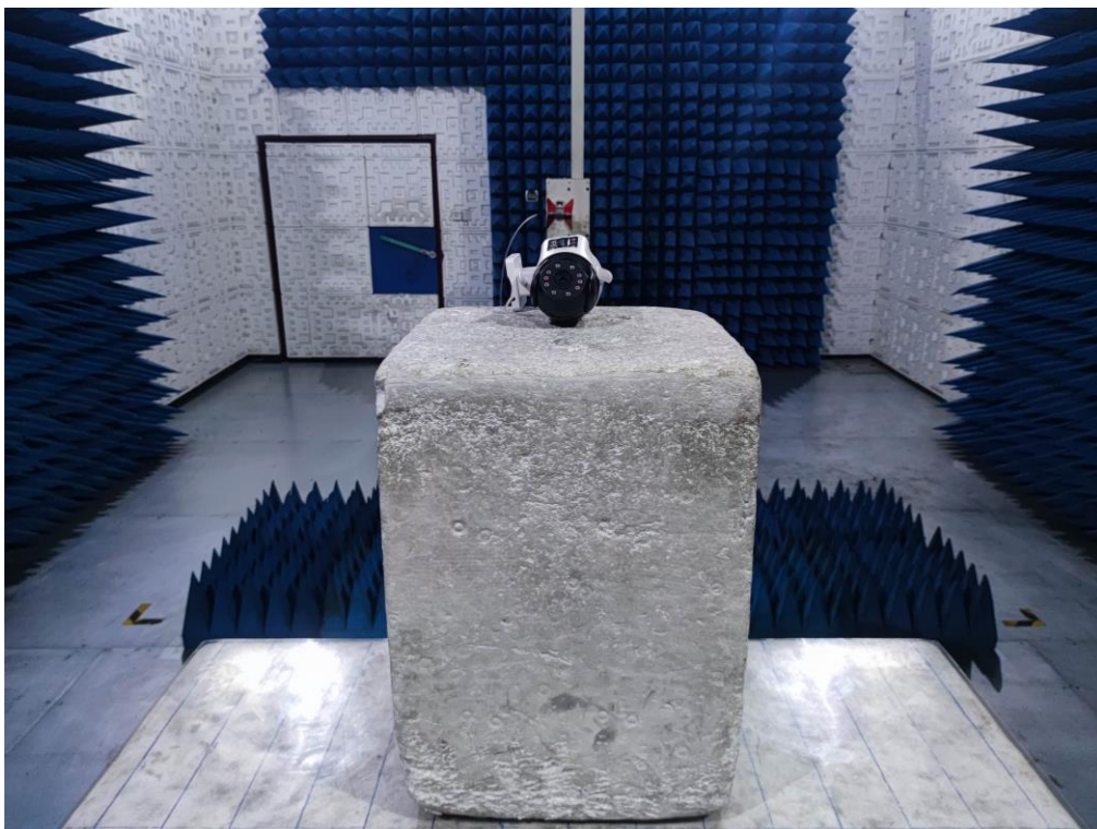
RADIATED EMISSION TEST SETUP ABOVE 1GHz
