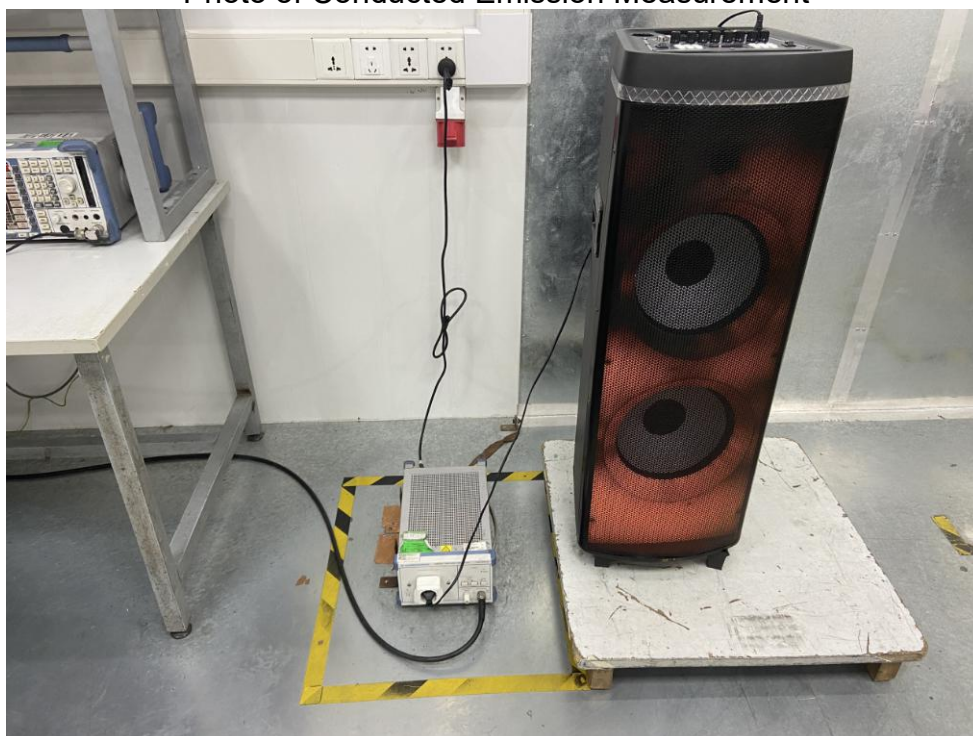
FCC ID: 2ANTA-UF-212E Photo of Conducted Emission Measurement
