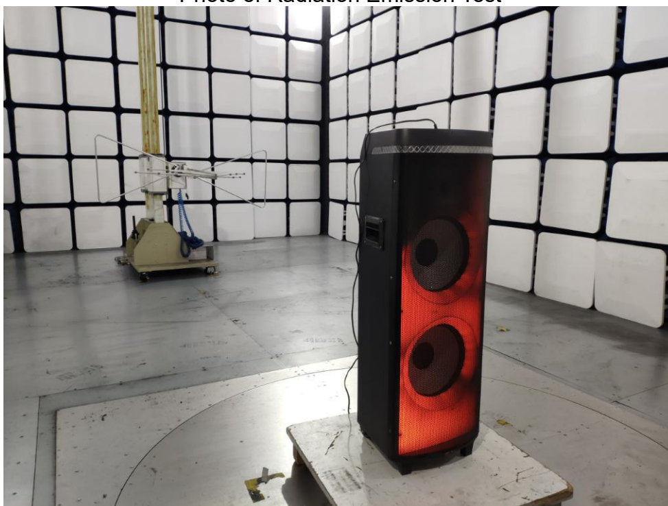
Photo of Radiation Emission Test
