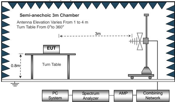
(C) Radiated Emission Test-Up Frequency Above 1GHz
