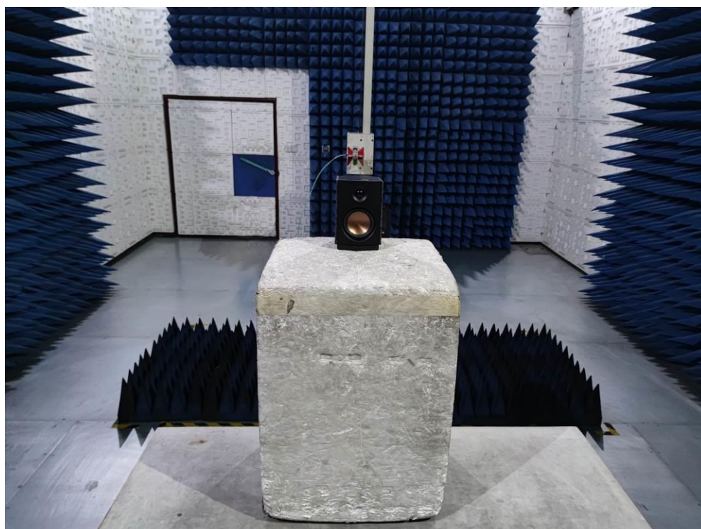
RADIATED EMISSION TEST SETUP ABOVE 1GHz
