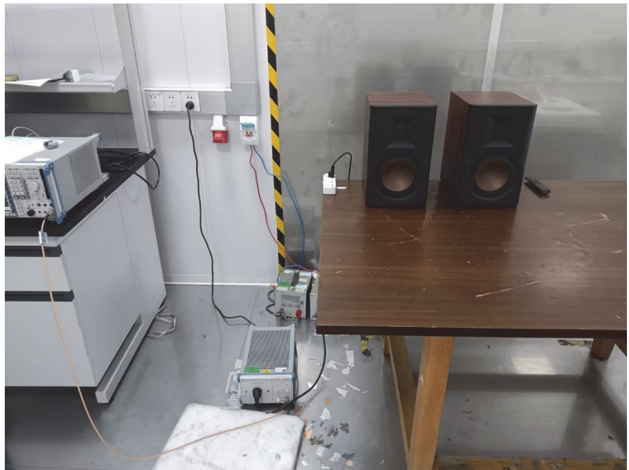
Conducted Emission Test Setup
