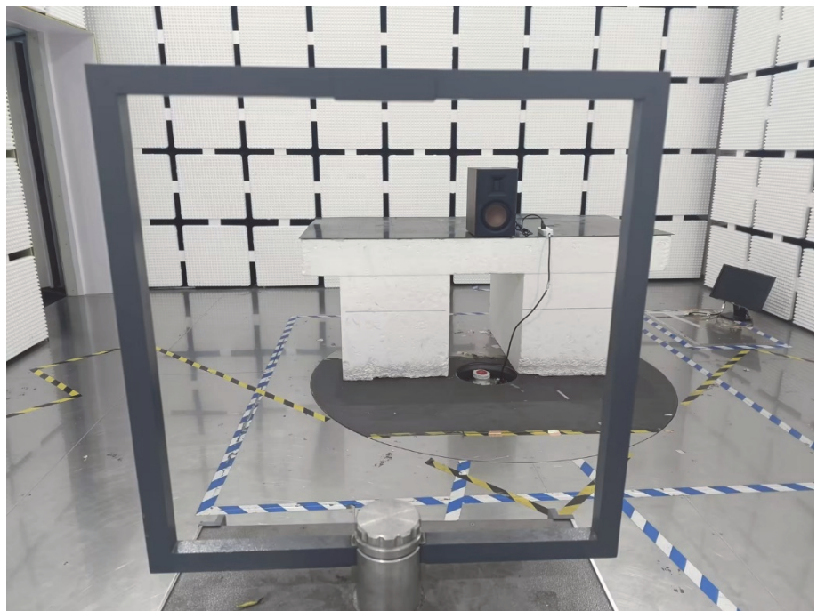
Radiation Emission Test Setup (Below 30MHz)
