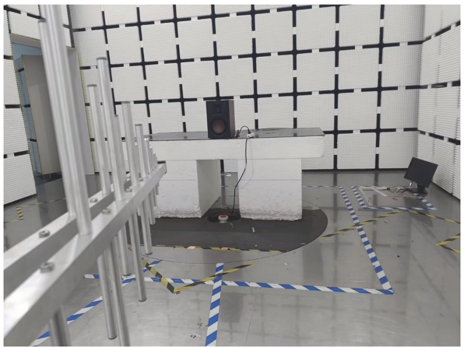
Radiation Emission Test Setup (30MHz to 1GHz)
