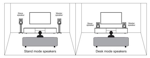
About the placement of stand mode speakers: When you need to put the speaker on a dedicated speaker stand, you should switch the selector switch of speaker's back panel to STAND mode.
