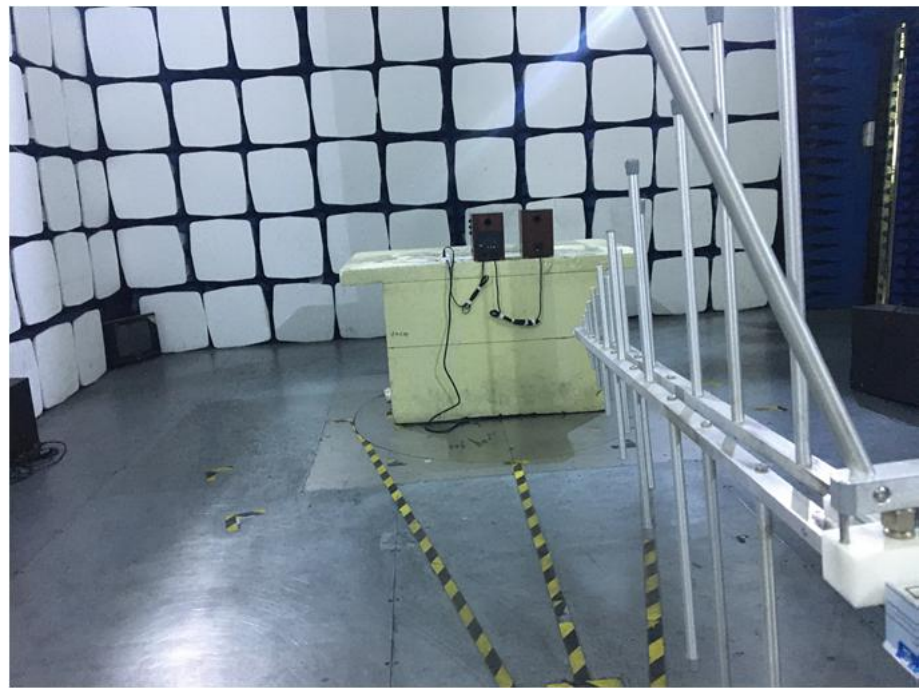
Radiation Emission Test Setup (30MHz to 1GHz)
