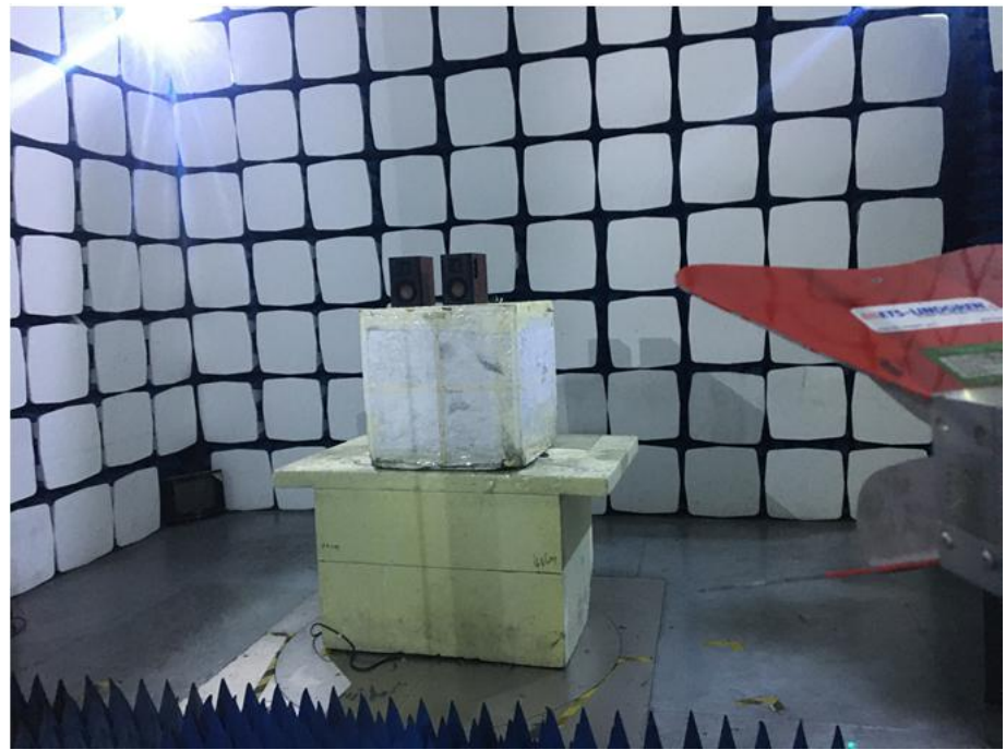
Radiation Emission Test Setup (1GHz to 18GHz)
