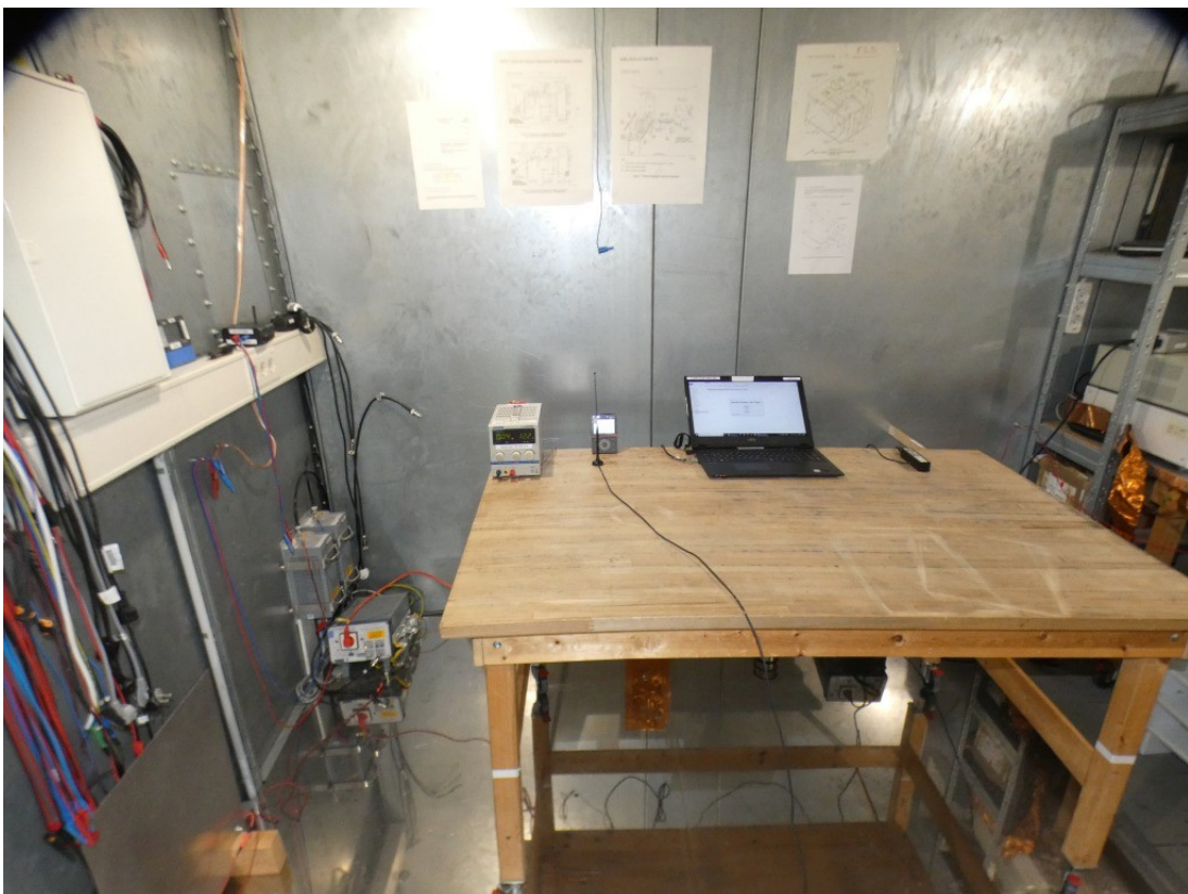
Photo 6: Test setup for conducted emissions FCC 15b
