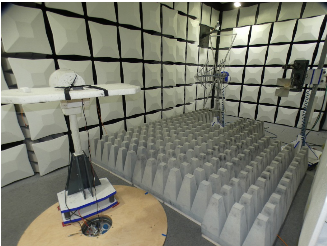
Photo 4: Test setup for radiated measurements above 1 GHz
