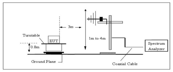
(B) Radiated Emission Test-Up Frequency Above 1GHz
