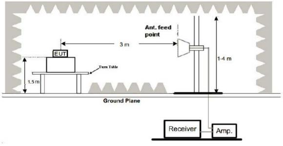
(3) Radiated Emission Test-Up Frequency Above 1GHz
