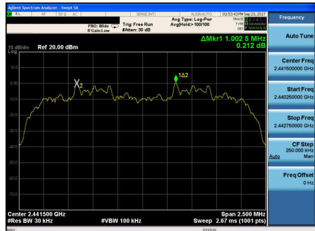
(2Mbps) Channel Separation plot on channel 39-40
