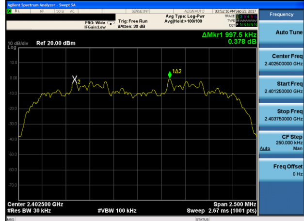
(2Mbps) Channel Separation plot on channel 39-40
