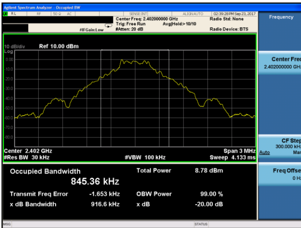
20dB Bandwidth plot on channel 39 (1Mbps)
