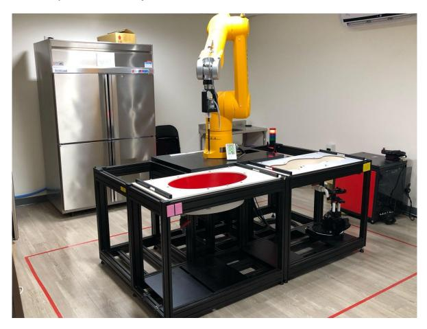
Liquid depth in the flat Phantom (≥15cm depth)
