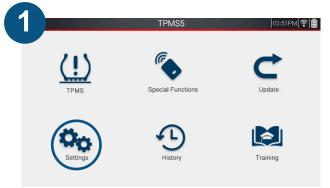
First, WiFi must be set up on the tool. select Settings.
