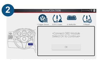
Continuing on to DTC Codes, ensure the OBDII Cable is connected to the tool and vehicle with the ignition in the ON position, Then tap "OK".
