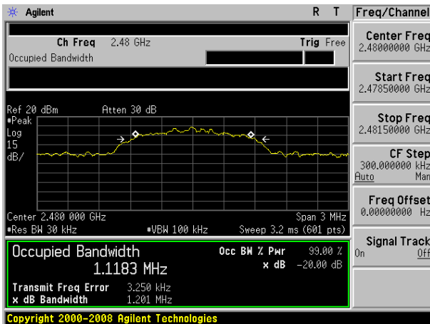
20dB Bandwidth plot on channel 78 (3Mbps)
