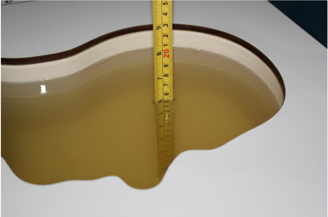
Picture 7-9: Liquid depth in the Head Phantom(2550MHz)
