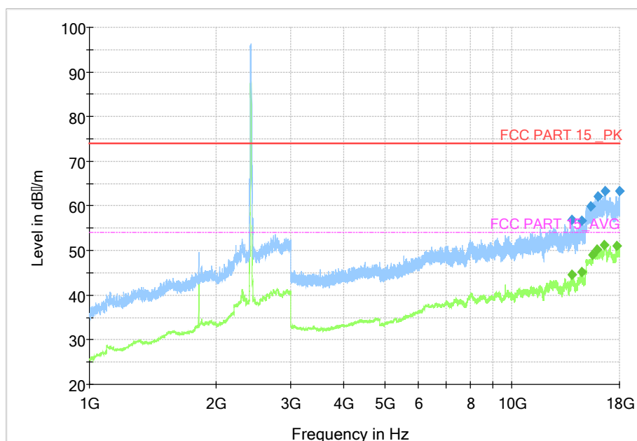
Fig.39 Radiated Spurious Emission (802.11g, CH1, 1 GHz-18 GHz)
