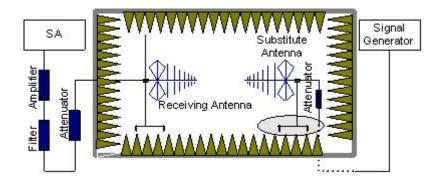
In the chamber, an substitution antenna for the frequency band of interest is placed at the reference point of the chamber. An RF Signal source for the frequency band of interest is connected to the substitution antenna with a cable that has been constructed to not interfere with the radiation pattern of the antenna. A power (P<sub>Mea</sub>) is applied to the input of the
