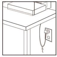
cord and coming in contact with the receptacle. If the plug or receptacle does get wet, DO NOT unplug the cord. Disconnect the fuse or circuit breaker that supplies power to the appliance. Then unplug and examine for presence of water in receptacle.
