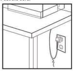
if an extension cord is used, to prevent water from travelling along the cord and coming in contact with the receptacle. If the plug or receptacle does get wet, DO NOT unplug the cord. Disconnect the fuse or circuit breaker that supplies power to the appliance. Then unplug and examine for presence of water in receptacle.
