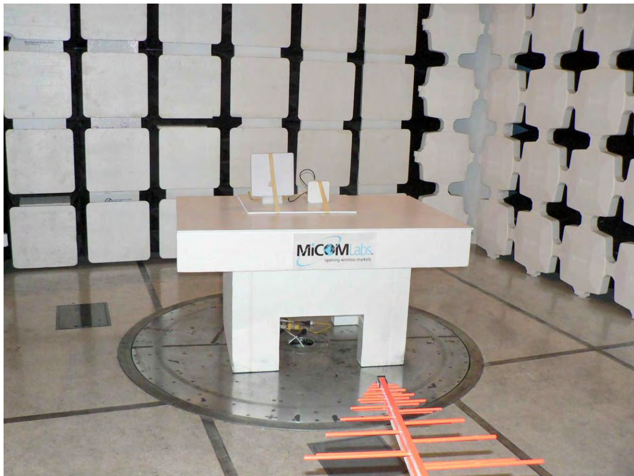
TIME01 EUT with ALR-A0501-F Antenna Transmitter Spurious 30-1000 MHz
