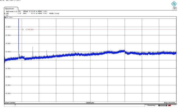
The peak above the limit is the carrier frequency.
