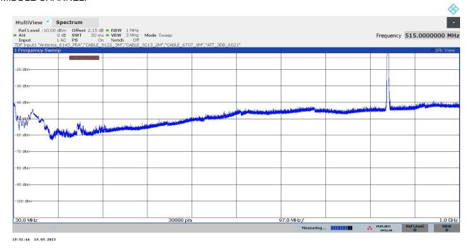
The peak above the limit is the carrier frequency: LTE Cat-M1 Band 26, 819 MHz
