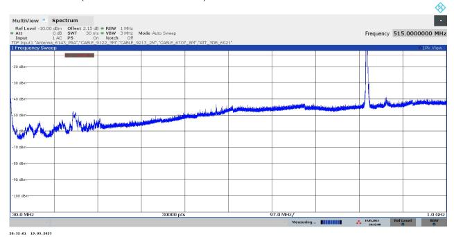
The peak above the limit is the carrier frequency: LTE Cat-M1 Band 26, 824 MHz
