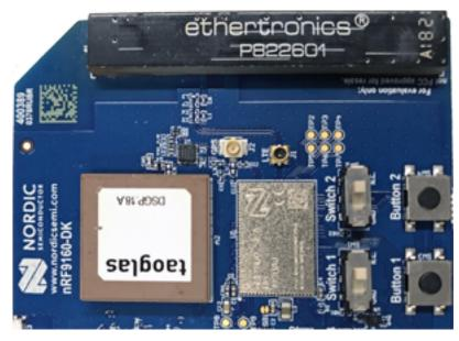
Figure 12: nRF9160 Development Kit antenna
