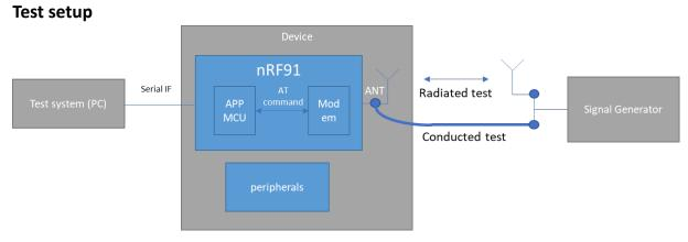
Figure 4: RX test setup example
