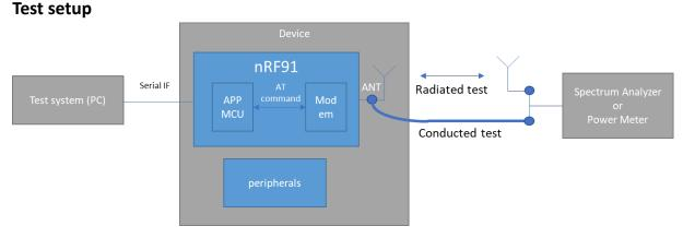
*Figure 6: TX test setup example*
