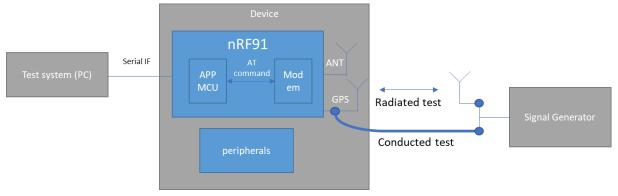
Figure 7: GPS SNR test setup example
