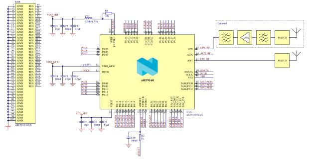
Figure 8: nRF9160 reference schematics
