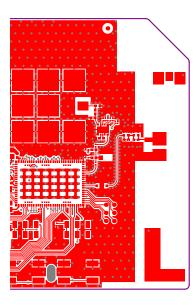
Figure 9: nRF9160 reference layout, metal layer 1 (top)
