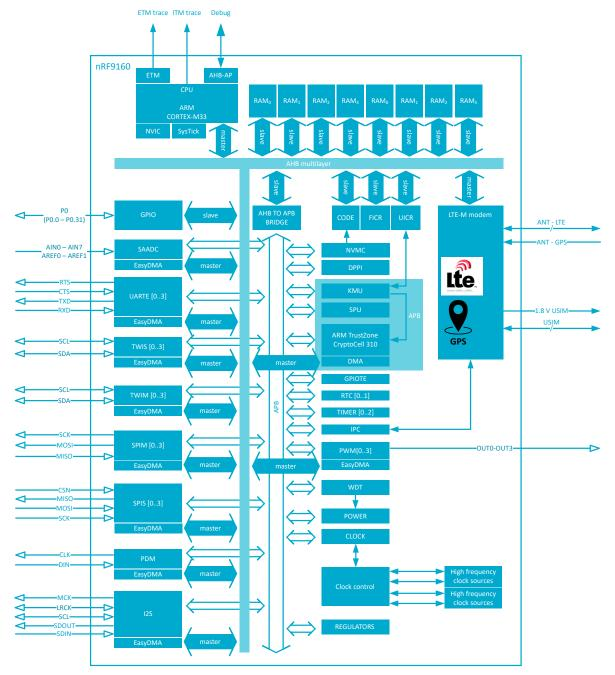
Figure 1: nRF9160 module block diagram
