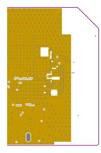
Figure 10: nRF9160 reference layout, metal layer 2
