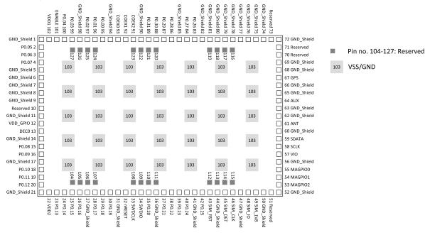
Figure 2: nRF9160 pinout, top (seen through module)
