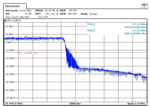
NOTE: The equipment transmits at the maximum output power
