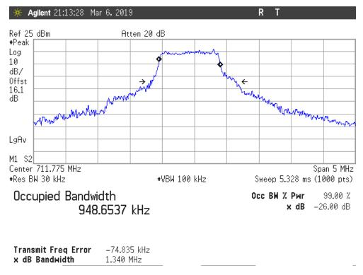
LTE QPSK MODULATION. BW = 5 MHz (Band 66)
