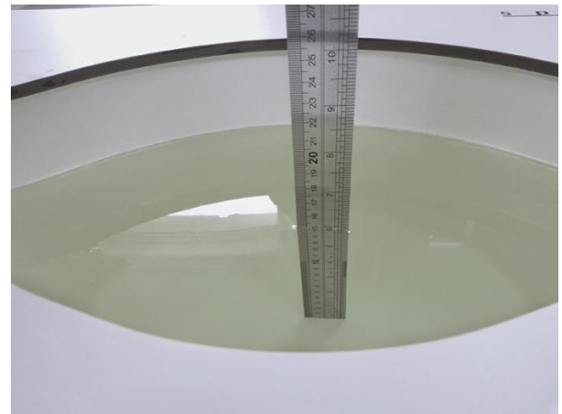
Liquid depth in the body phantom (2450MHz)
