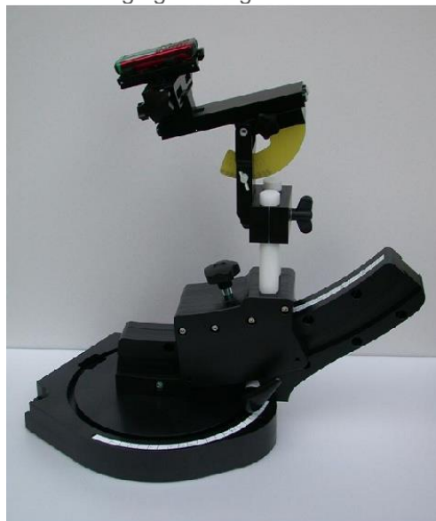
Device holder supplied by SPEAG
