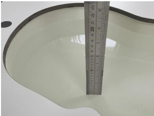
Liquid depth in the head phantom (2450MHz)
