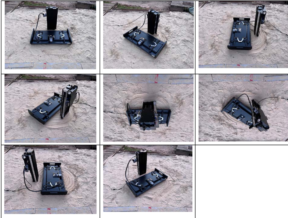
EUT Positions with 45 Degree Interval
