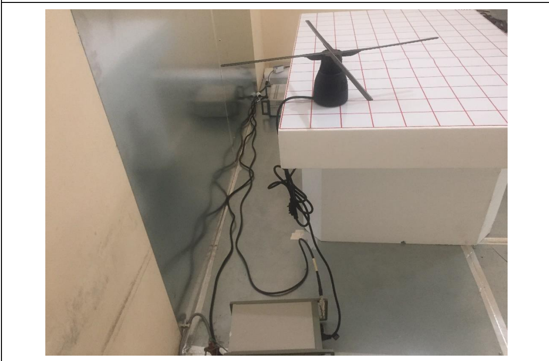
AC Line Conducted Emission setup – Rear
