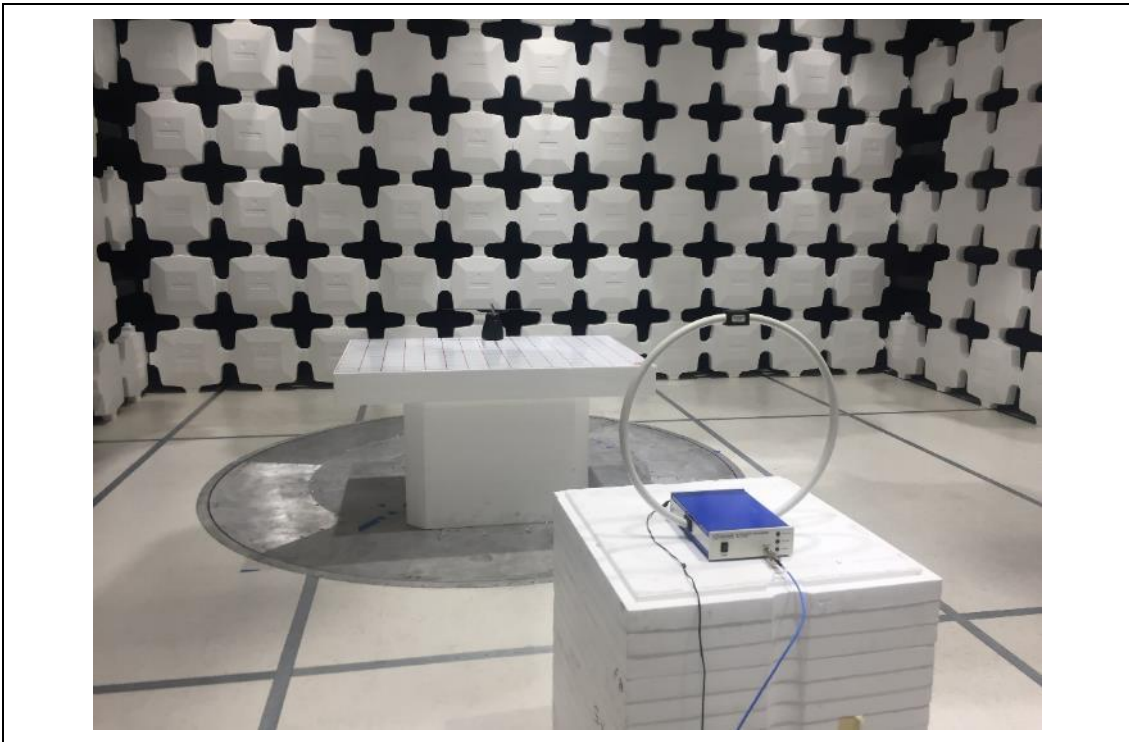
Radiated Emissions Below 30MHz setup – Front
