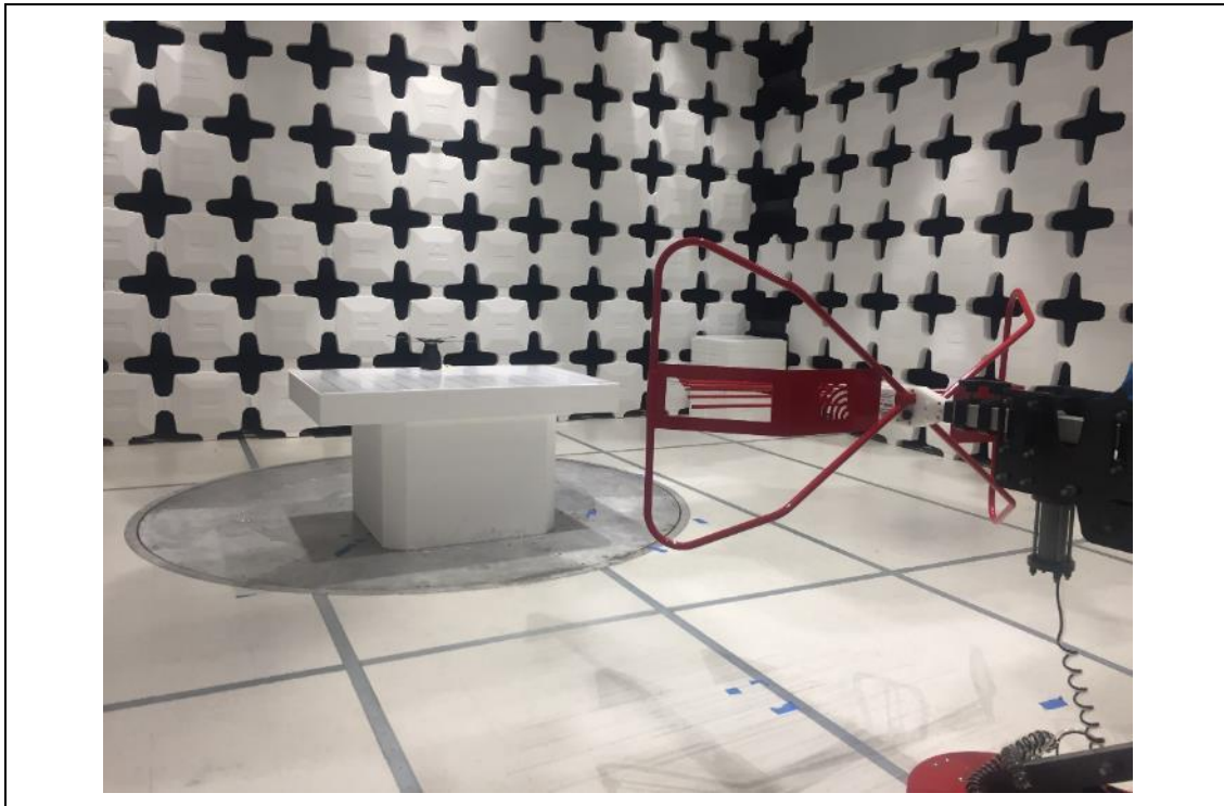
Radiated Emissions Below 1GHz setup – Front
