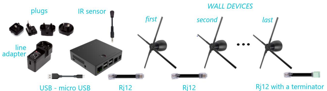
Picture 8. Connection scheme
