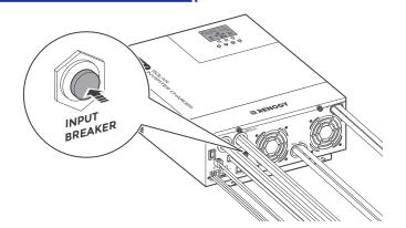
The inverter charger provides an input breaker that automatically pops up when the AC input current is higher than 40A. This helps cut off the AC input and prevent the inverter charger from being damaged.
