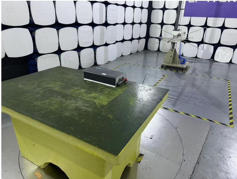
Spurious Emission Test Setup (Below 1GHz)
