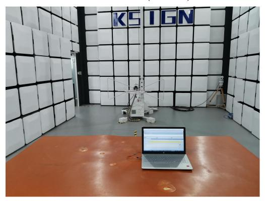
Radiated Measurement (Above 1GHz)
