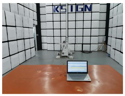
Radiated Measurement (Above 1GHz)
