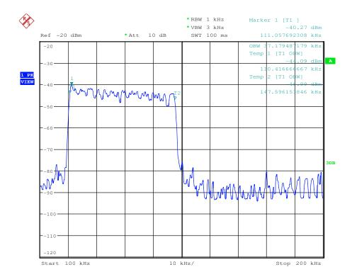
According the test data above, the fundamental wave is not fall in the restricted band 90KHz-110KHz, the field strength also meet the 15.209 requirement, please refer to clause 7.4.
