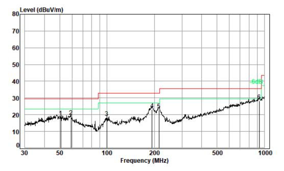
Condition: 10m HORIZONTAL Job No. : 19045CR Test Mode: a
