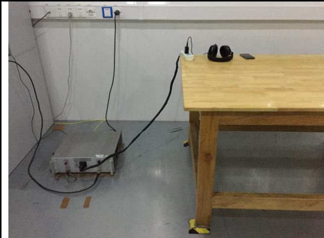
Conducted Emissions Test Setup Front View
