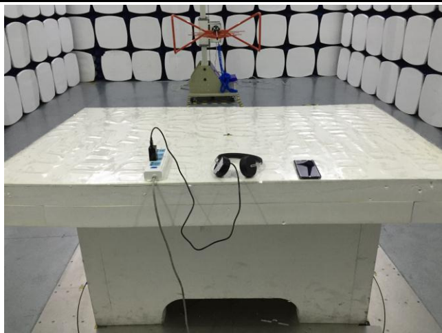
Conducted Emissions Test Setup Front View
