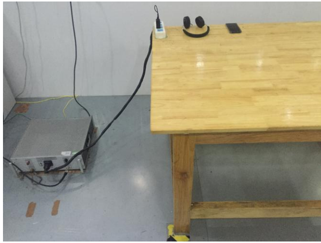
Conducted Emissions Test Setup Front View
