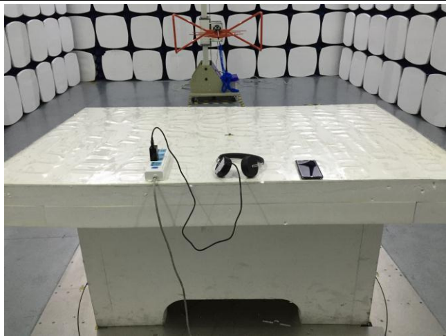
Conducted Emissions Test Setup Front View
