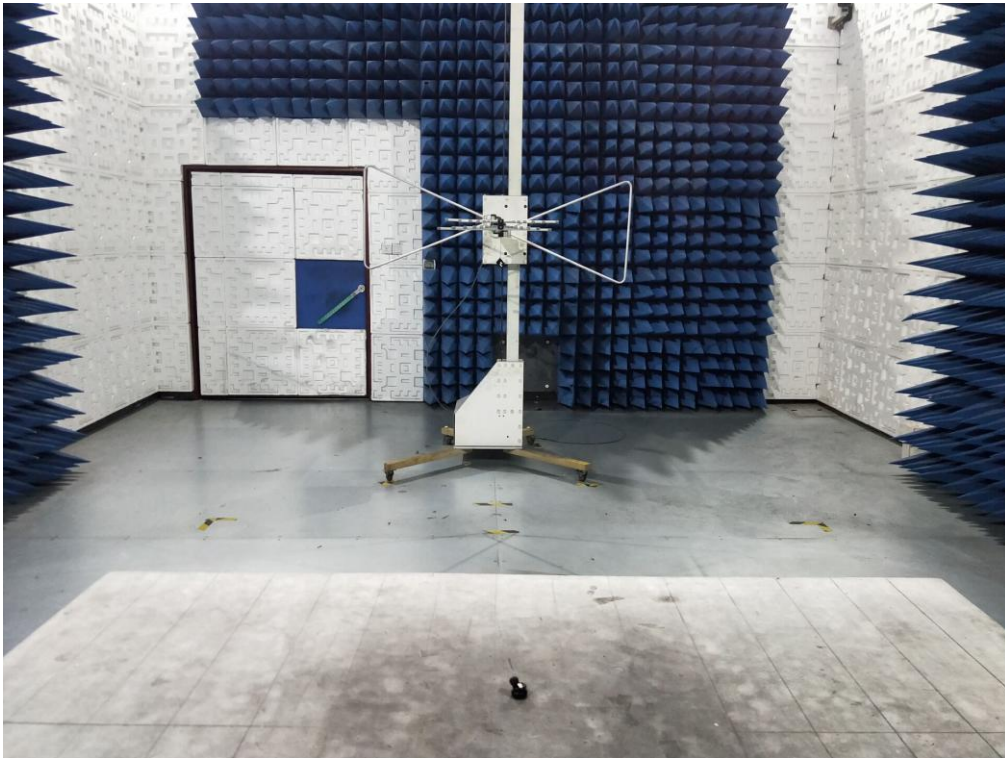
RADIATED EMISSION TEST SETUP ABOVE 1GHZ
