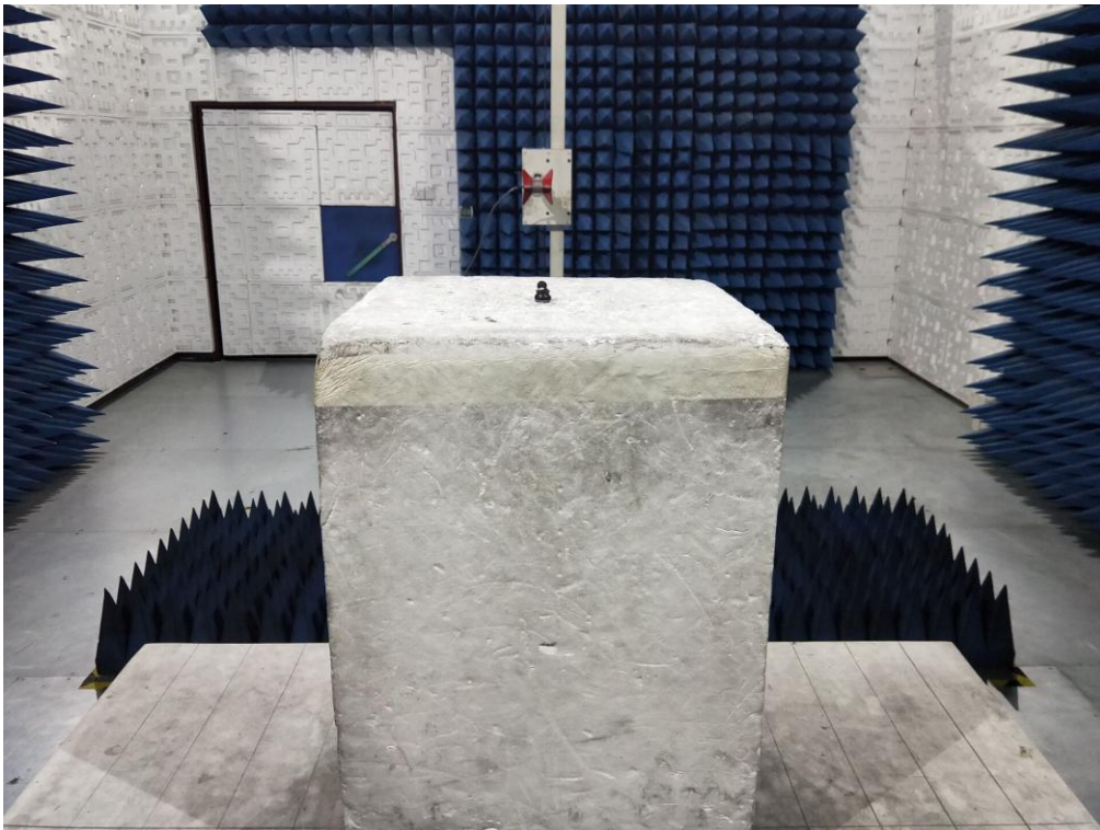
RADIATED EMISSION TEST SETUP ABOVE 1GHZ
