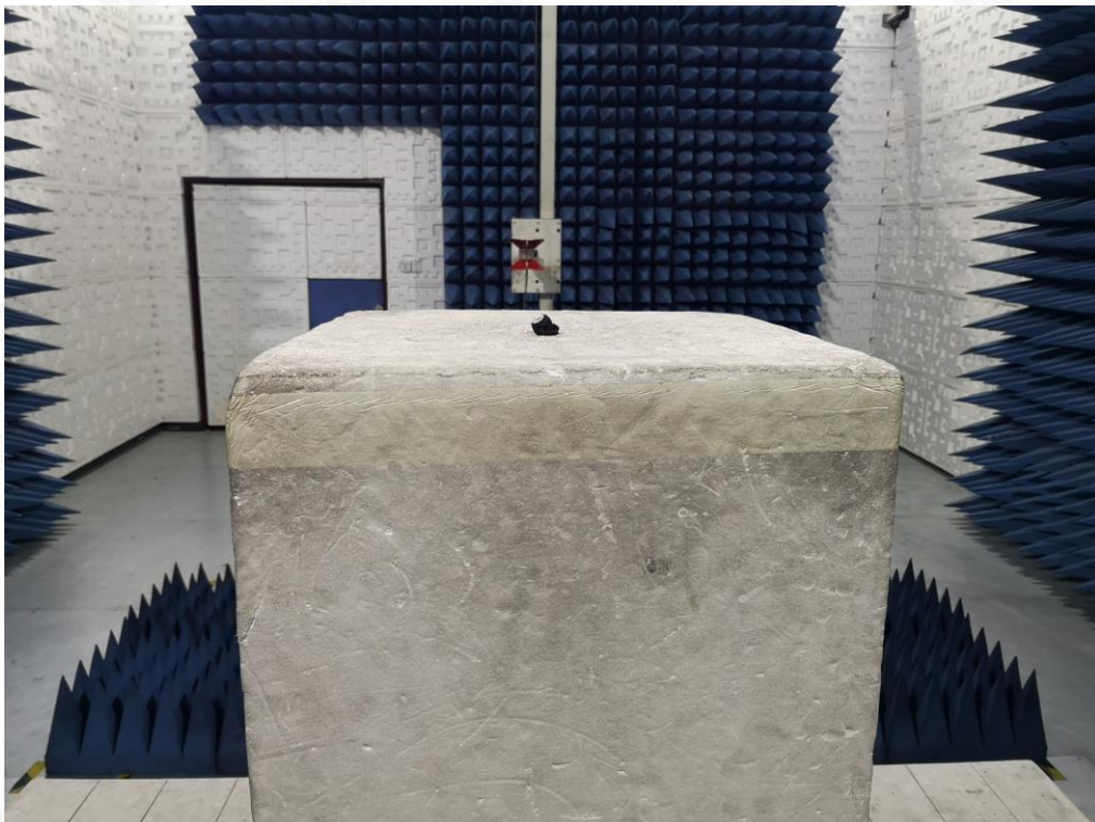
RADIATED EMISSION TEST SETUP ABOVE 1GHZ
