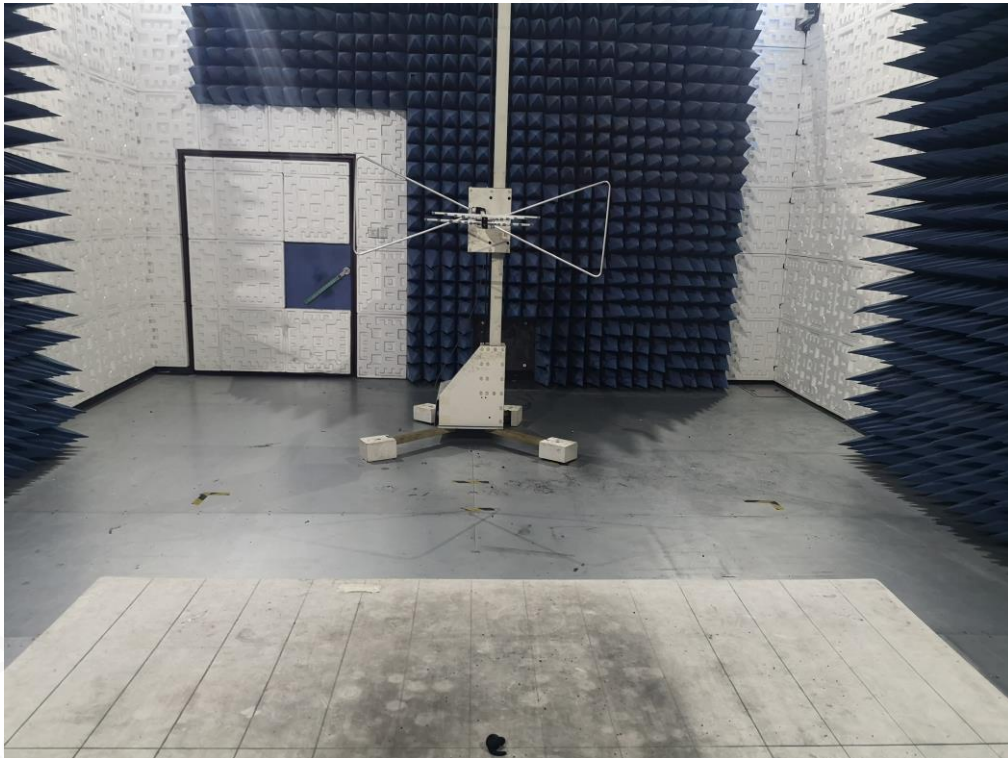
RADIATED EMISSION TEST SETUP ABOVE 1GHZ
