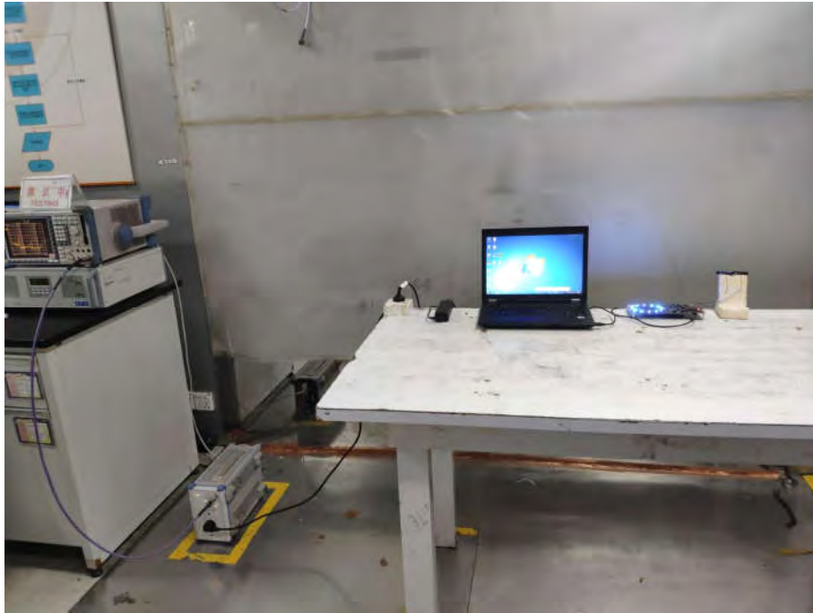
Conducted Emissions Test Setup
