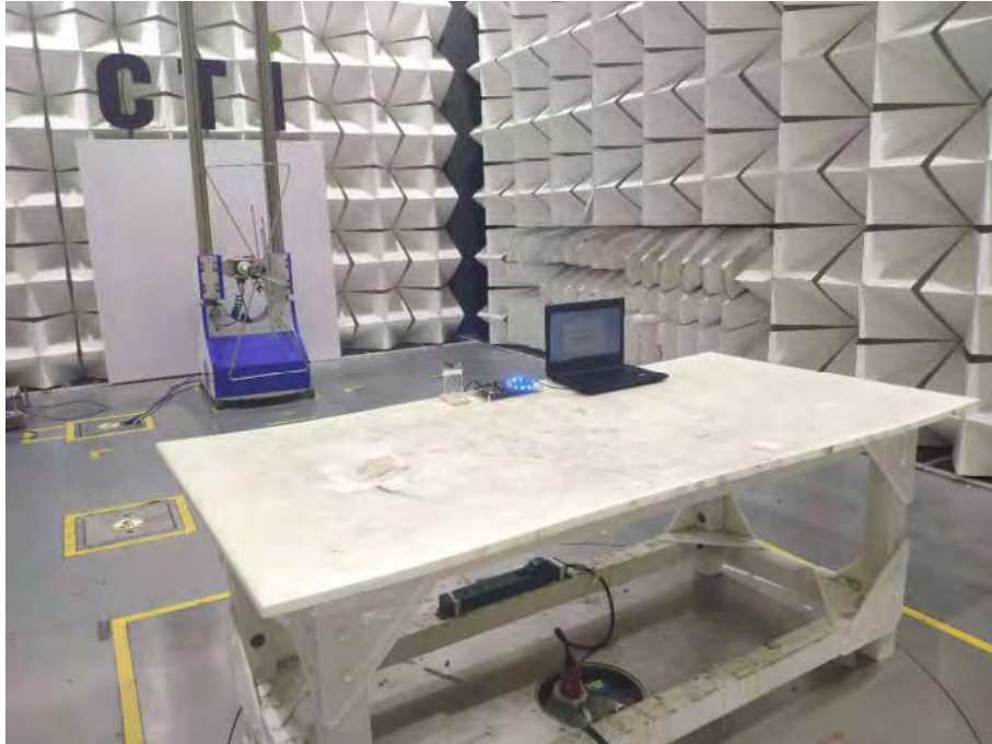
Radiated spurious emission Test Setup-1(Below 1GHz)
