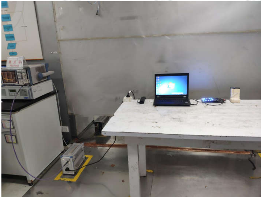
Conducted Emissions Test Setup
