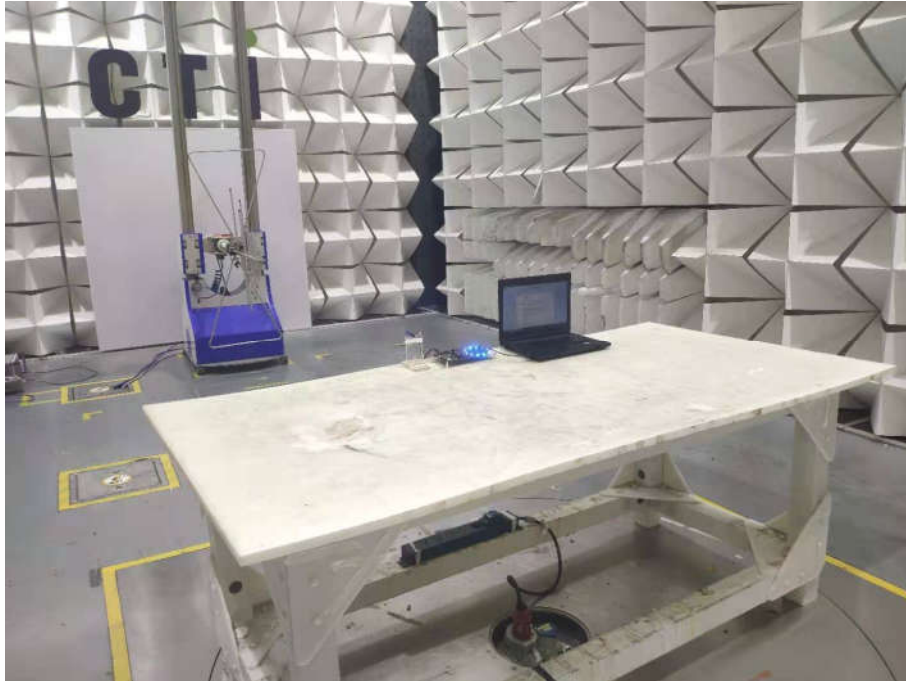
Radiated spurious emission Test Setup-1(Below 1GHz)
