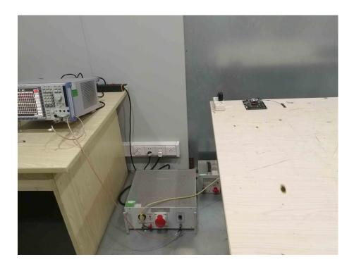
Radiation Emission Test Setup (Below 30MHz)
