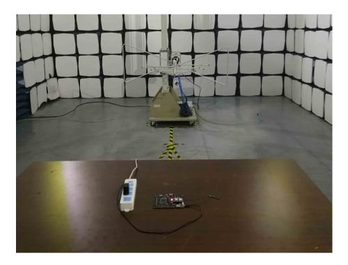
Radiation Emission Test Setup (Above 1GHz)
