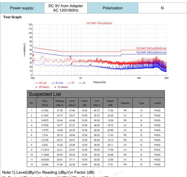
2). Factor (dB)=insertion loss of LISN (dB) + Cable loss (dB)
