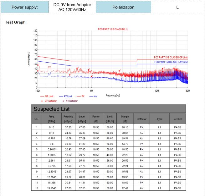
Note:1).Level( $dB\mu V$ )= Reading ( $dB\mu V$ )+ Factor (dB)
