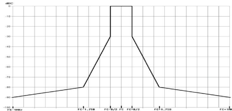
Figure 4: Spectrum mask for digital systems below 1 GHz
