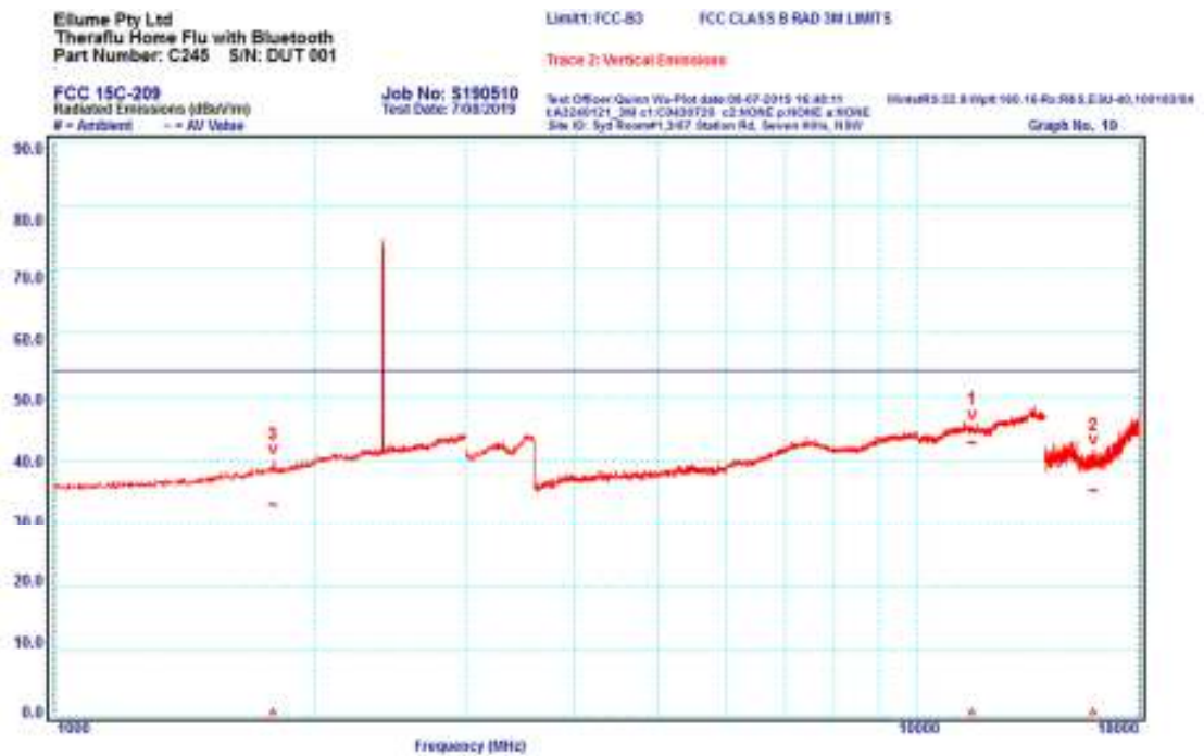
Graph 19 Vertical Polarisation 1000 to 18000 MHz
