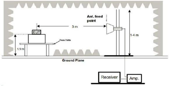
(3) Radiated Emission Test-Up Frequency Above 1GHz
