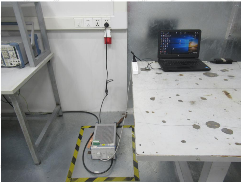
Photo of Conducted Emission Measurement
