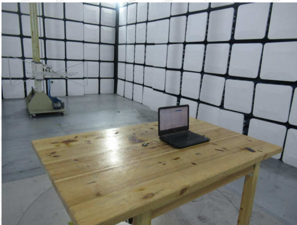
Photo of Radiation Emission Test
