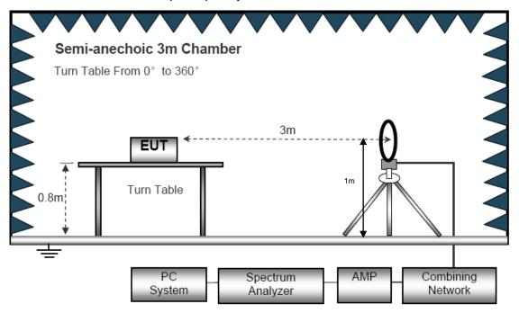
(B) Radiated Emission Test-Up Frequency 30MHz~1GHz
